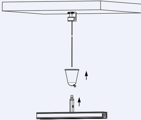
**Step 4-2: Fix the ceiling cup with screws.**
