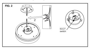
3. First keep the two buckle lugs in the gap on the mounting disc. And put the guide post in the center of the lamp body to the convex hole on the mounting plate, keep the center position consisten, and then push up the lamp body flat. Finally rotate the lamp body to the right and lock the light.
