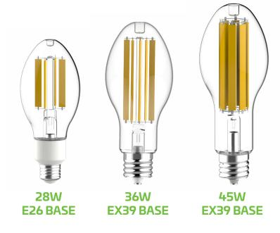
Filament-style LED lamp designed to replace up to 175W metal halide and 150W high pressure sodium lamps
