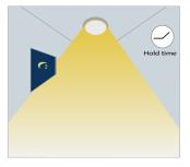
Light dims to stand-by level (10%, 20%, 30% or 50%) if no motion is detected after holdtime.
