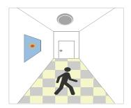
With sufficient ambient brightness, the light remains OFF when motion is detected.
